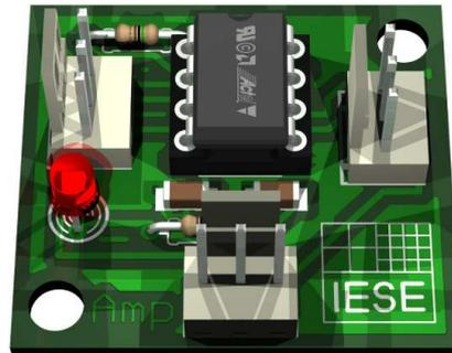
Figure 5.6.: Instrumentation amplifier printed circuit board
