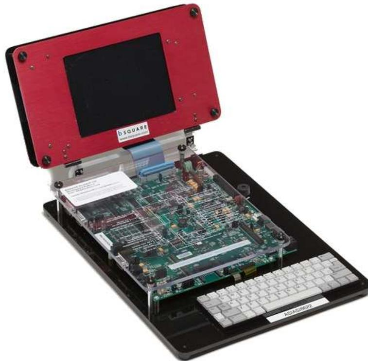
Figure 5.2.: DevkitIDP development board based on the Intel PXA255 Application Processor
